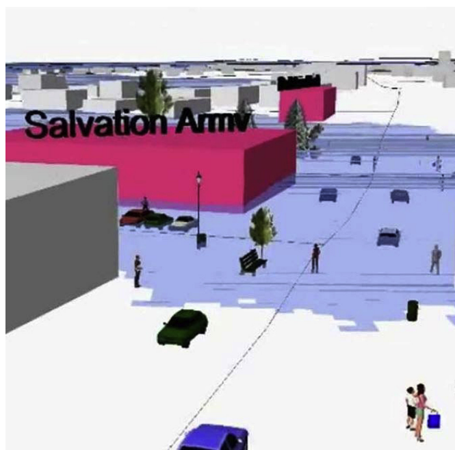
Fig. 3. Three-dimensional visualization of the probable worst-case flood depth for a 1-in-10 year, 8.9 m flood event (CGVD28 datum) affecting the downtown core of Sackville, New Brunswick (reprinted with permission from Geomatica 66: 255–265, published by the Canadian Institute of Geomatics).
