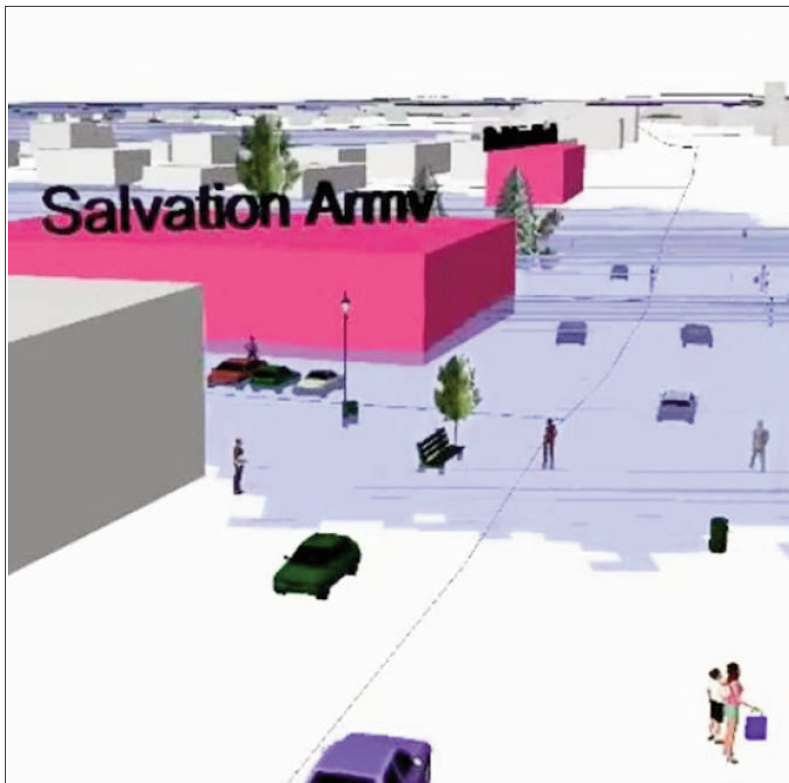
Figure 6: “Walking man” animation illustrating the potential consequence of a 1-in-10 year flood event of 8.9m (CGVD28 datum, R.J. Daigle Enviro [2011]) in downtown Sackville, New Brunswick. In this context, 3D visualization facilitates an awareness of flood depth and severity (e.g., where cars are fully vs. only partially submerged) in a familiar setting, and may be more emotionally compelling.
