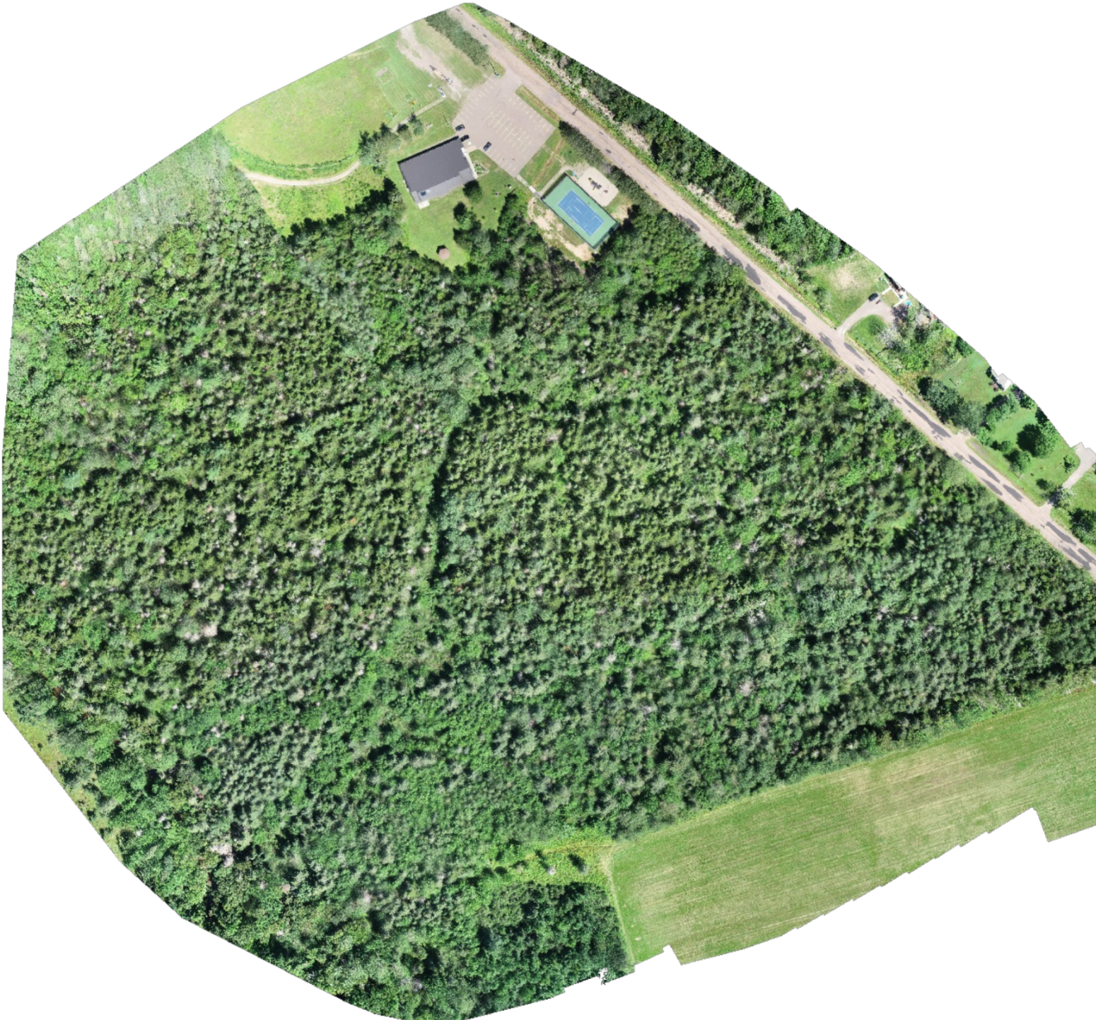
The orthomosaic created by the author in August of 2022 of the property in Cormier-Village. The building to the top left next to the tennis court is the community center. Although not perfect, it does provide a visual model of the property. It would also be used as a comparative model to our post-hurricane assessment.
